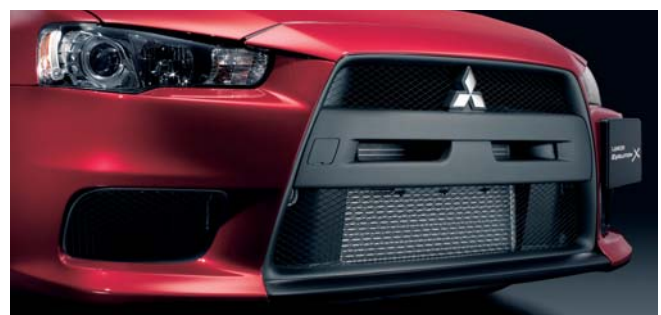
Thermoplastic resin bumper on the Lancer Evolution X
