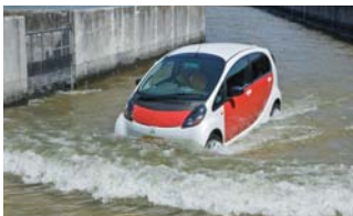
Water-crossing test at 30 cm depth
