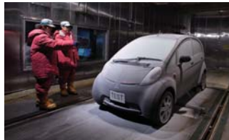
Cold-weather testing at minus 15°C
