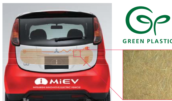
Green Plastic applications: Interior parts made from bamboo fiber in an i MiEV research vehicle (fleet monitor)
